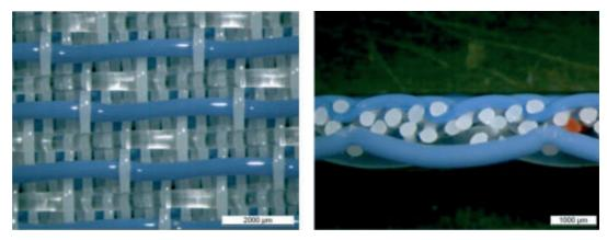
**Figure 12**. shows the unique machine side interlacing pattern which a) exposes the entire diameter of the roll side yarns to sacrificial wear, and b) reduces overall contact area with stationary objects to reduce sliding friction.
