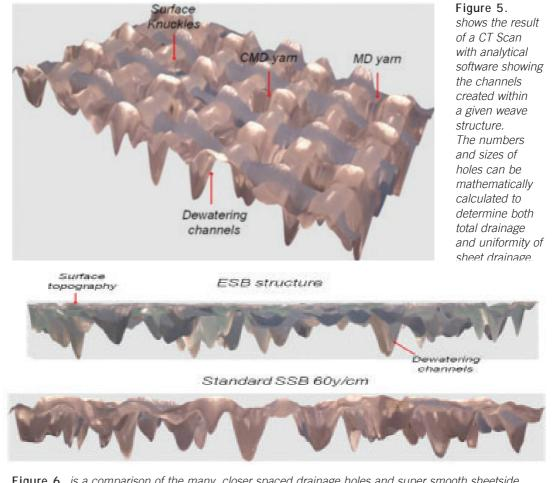
**Figure 6**. *is a comparison of the many, closer spaced drainage holes and super smooth sheetside topography of the ESB, compared to the SSB style of forming fabric which has been considered state-of-the-art for the last 5 years. The more infrequent, larger holes in older SSB structures induce the migration of fines and fillers toward the holes.*
