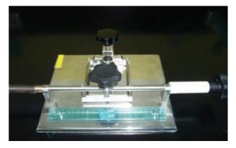
**Figure 9**. compares diagonal distortion. A fabric sample is clamped in place, sideways force is applied, and the distance that the fabric deflects is measured.
