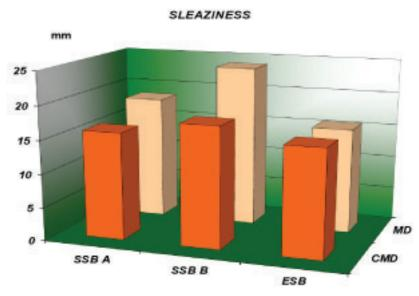
**Figure 10**. shows the result of comparing two of the most common SSB designs to the ESB. Smaller numbers mean less deflection and higher stability.
